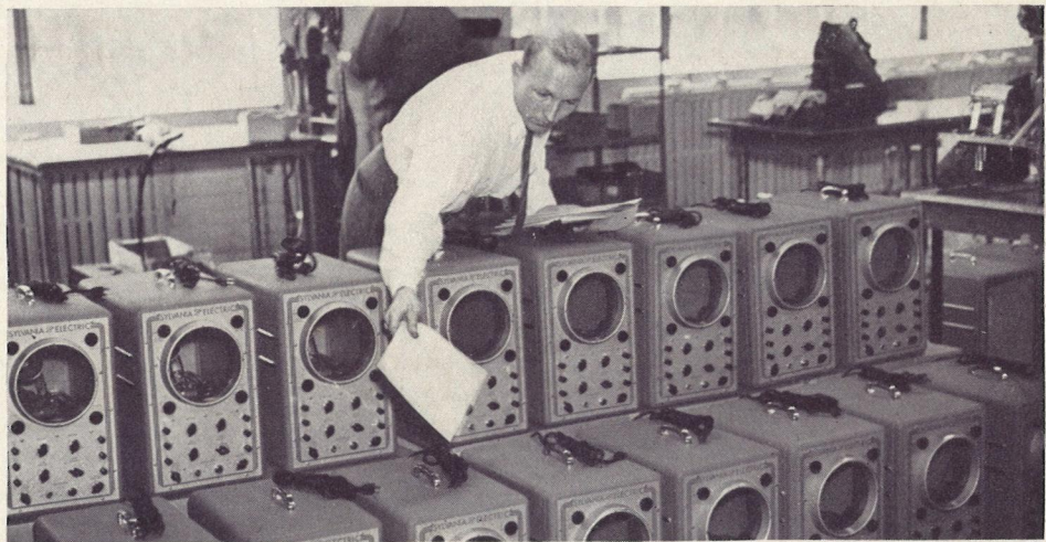
NOW BILL THOMAS gives the completely assembled instrument a final check before cabinet assembly. All tests used in radio servicing are simulated in final check of the instrument.
